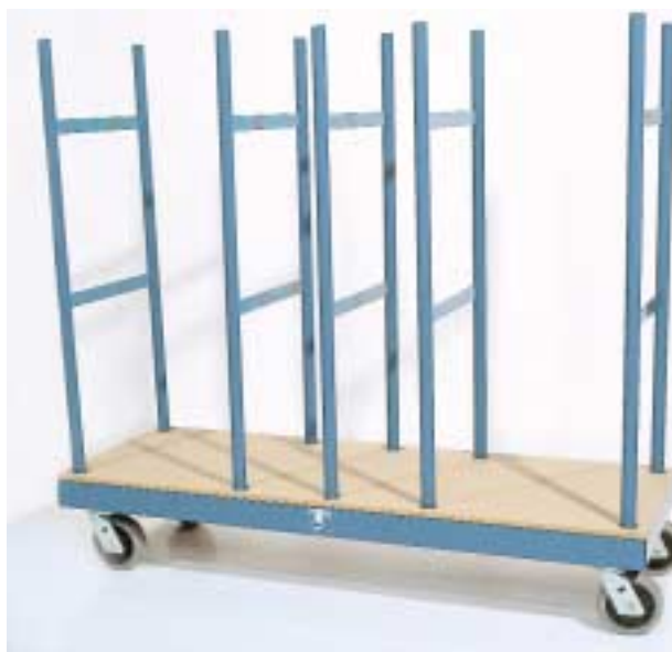
A lateral cart, like the one shown on the right from ShopCarts USA, allows panels to be arranged vertically, making them easier to access; ShopCarts USA’s Panel Handler can transport sheet stock vertically, and then be tilted flat to function as an infeed table at a machine.
