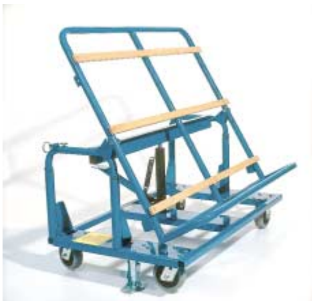
A lateral cart, like the one shown on the right from ShopCarts USA, allows panels to be arranged vertically, making them easier to access; ShopCarts USA’s Panel Handler can transport sheet stock vertically, and then be tilted flat to function as an infeed table at a machine.
